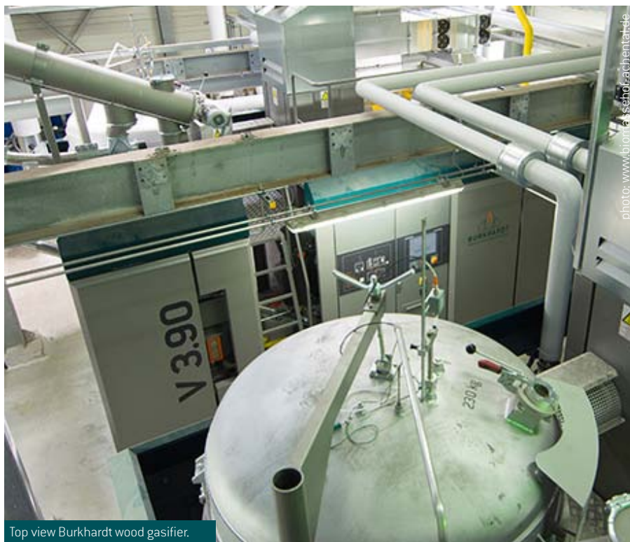
After modification: now two Burkhardt Gasifiers supply one CHP
